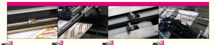
QSA-dies (quick size adjustment) allow for quick and simple deselection of punching pins. Re-collating station.
